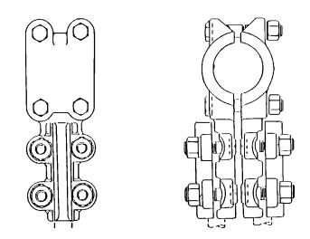
Bronze Alloy Tee for Copper Pipe Main to (2) Copper Cable Taps.
