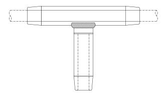
\*ATCC-EHV" is a streamlined, tapered cable to cable Aluminum compression tee for use on EHV applications for Corona-free service.
