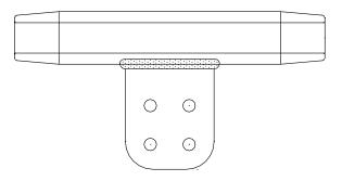
Type ATCF-EHV" compression tee to flat. Used for EHV applications where streamlined, tapered connectors are needed for corona free service. Add "EHV" to standard catalog number. EX: ATCF-1031-4B-EHV. See compression section page 281.
