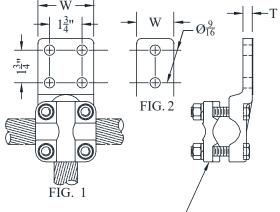
CAP MAY BE TURNED OR REVERSED TO CLAMP CONDUCTOR WITHIN RANGE SHOWN.
